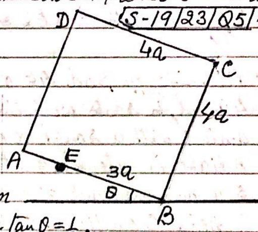
4. A uniform square lamina ABCD of side  $4a$  and weight  $W$  rests in a vertical plane with the edge AB inclined at an angle  $\theta$  to the horizontal, where  $\tan \theta = \frac{1}{3}$ . The vertex B is in contact with a rough horizontal surface for which the coefficient of friction is  $\mu$ . The lamina is supported by a smooth peg at the point E on AB, where  $BE = 3a$ .
