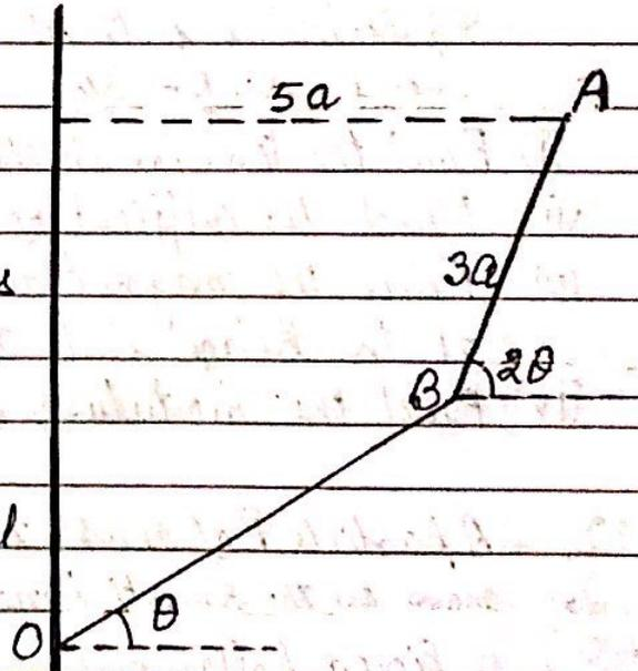
The string and the rod make angles  $\theta$  and  $2\theta$  respectively with the horizontal. The system is in equilibrium with the rod and the string in the same vertical plane. It is given that  $\sin \theta = \frac{3}{5}$  and you may use the fact that  $\cos 2\theta = \frac{7}{25}$ .
