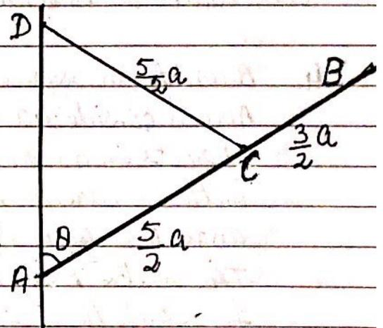
3. A uniform rod AB of length  $2a$  and weight  $W$  rests on the smooth rim of fixed hemispherical bowl of radius  $a$ . The end B of the rod is in contact with the rough inner surface of the bowl. The coefficient of friction between the rod and the bowl at B is  $\frac{1}{3}$ . (continued  $\rightarrow$ )
