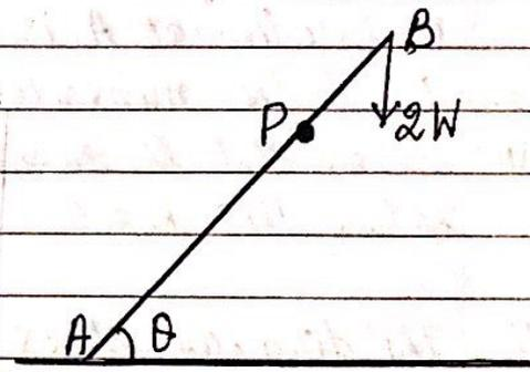
The system is in limiting equilibrium with the angle between the rod and the horizontal surface equal to  $\theta$ , where  $\tan\theta = \frac{4}{3}$ . The coefficient of friction between the rod and the surface is  $\frac{2}{3}$ . Find the distance AP. [S-16/23/Q2] --- [8]
