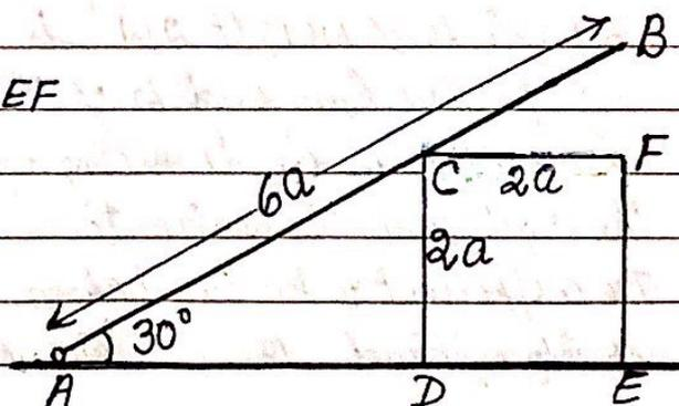
uniform rod AB, of weight  $W$  and length  $6a$ , is hinged to the plane at A. The rod rests in smooth contact with the cube at C, with angle CAD equal to  $30^\circ$ . The rod is in the same vertical plane as CDEF. The coefficient of friction between the plane and the cube is  $\mu$ . Given that the system is in equilibrium, show that  $\mu \geq \frac{3}{25}\sqrt{3}$  ---[6]
