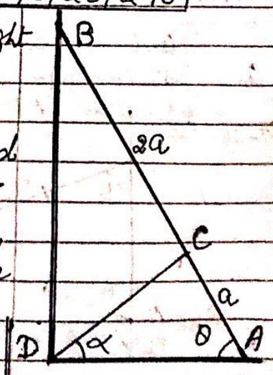
equilibrium in a vertical plane perpendicular to the wall with the ladder making an angle  $\theta$  with the horizontal and the rope making an angle  $\alpha$  with the horizontal. It is given that  $\tan \theta = 2 \tan \alpha$ . (Continued  $\rightarrow$ )
